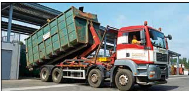
When full, the containers can be removed from ground level by hooklift trucks without having to close the site to public on the deck level.
